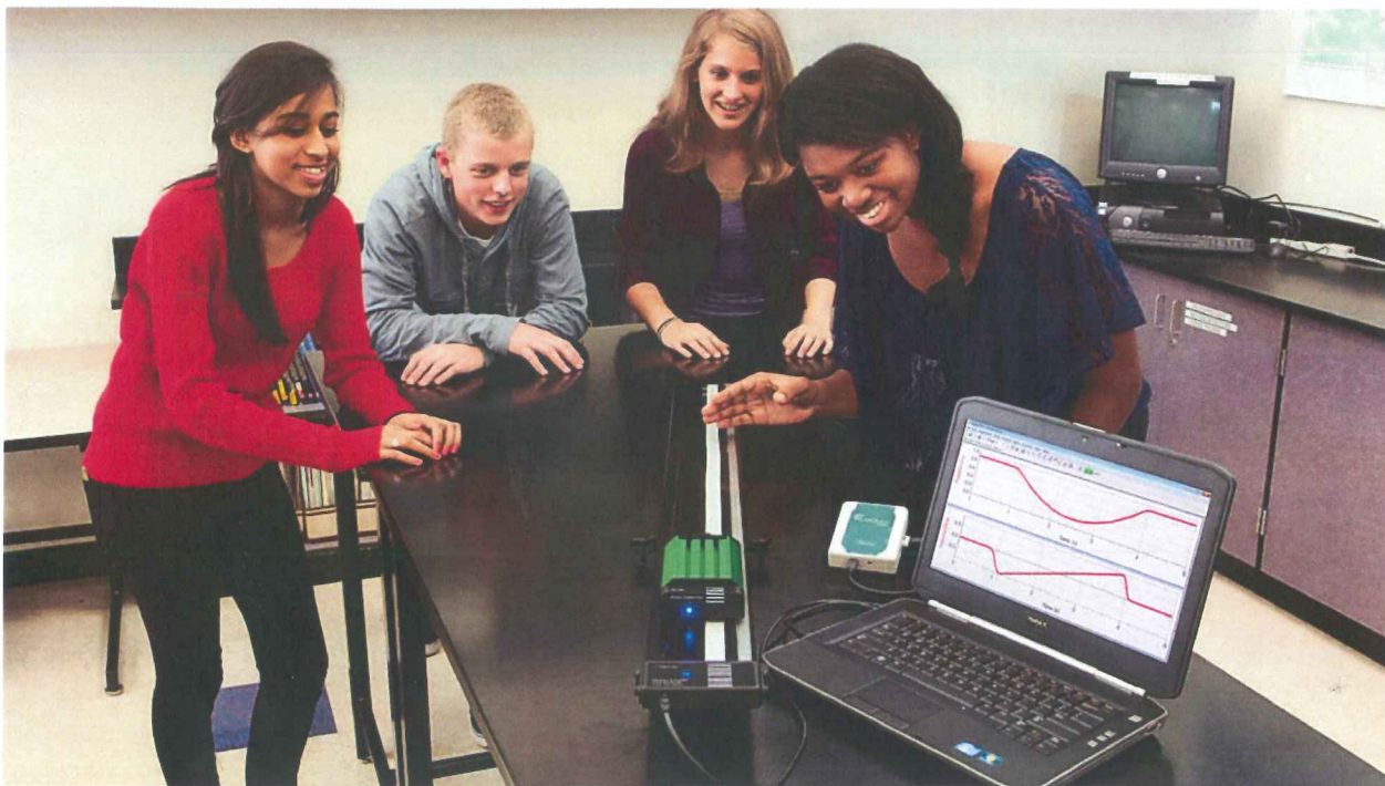
Students using the Vernier Motion Encoder System. The computer display show distance vs. time and velocity vs. time graphs.
